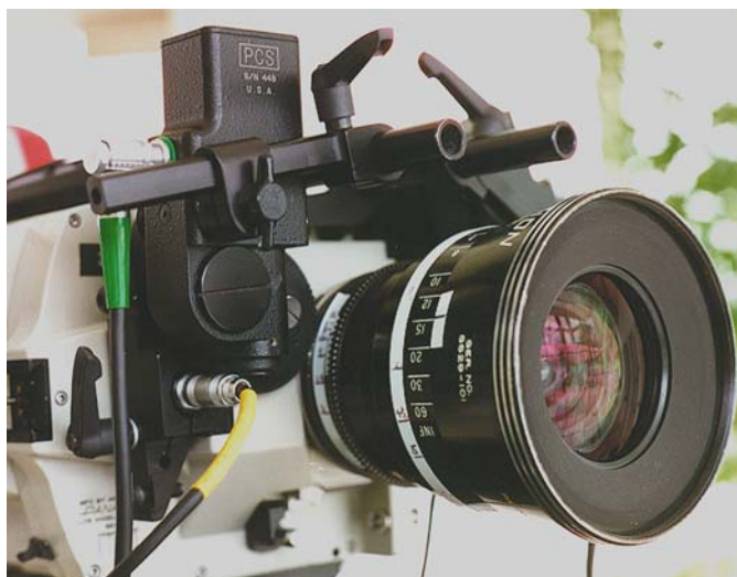
Hill Pana Bracket and PAM motor mount on Panavision camera
