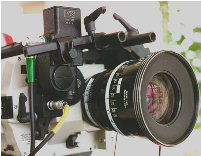
Panavision camera with Hill Pana bracket and PAM Mount.
