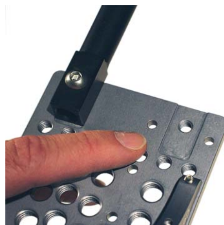
The top cheese plate will have two notches for the Hill square to round rods (15mm) for motor placement.
